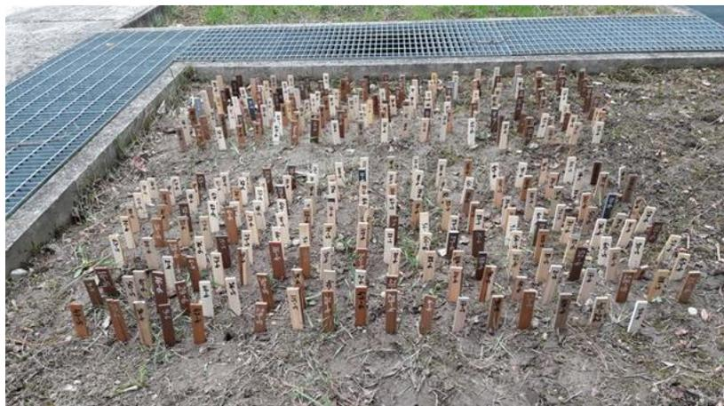
*Figure 3: Facades materials during degradation in soil – simulation of landfilling*
