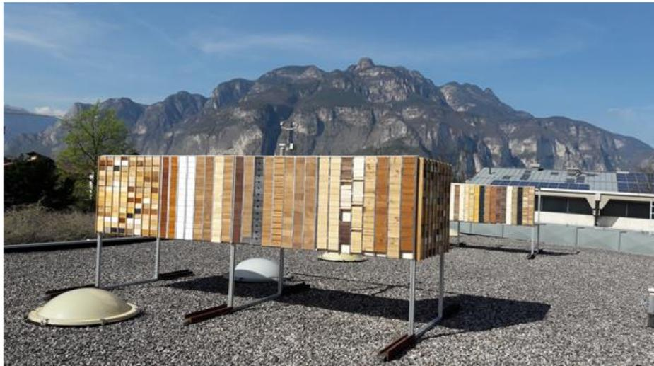
*Figure 1: Facades materials exposed to natural weathering*
