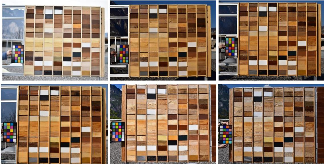
*Figure 2: Facades materials at the beginning of weathering test, and their appearance with the progress of weathering (up to 5 months).*
