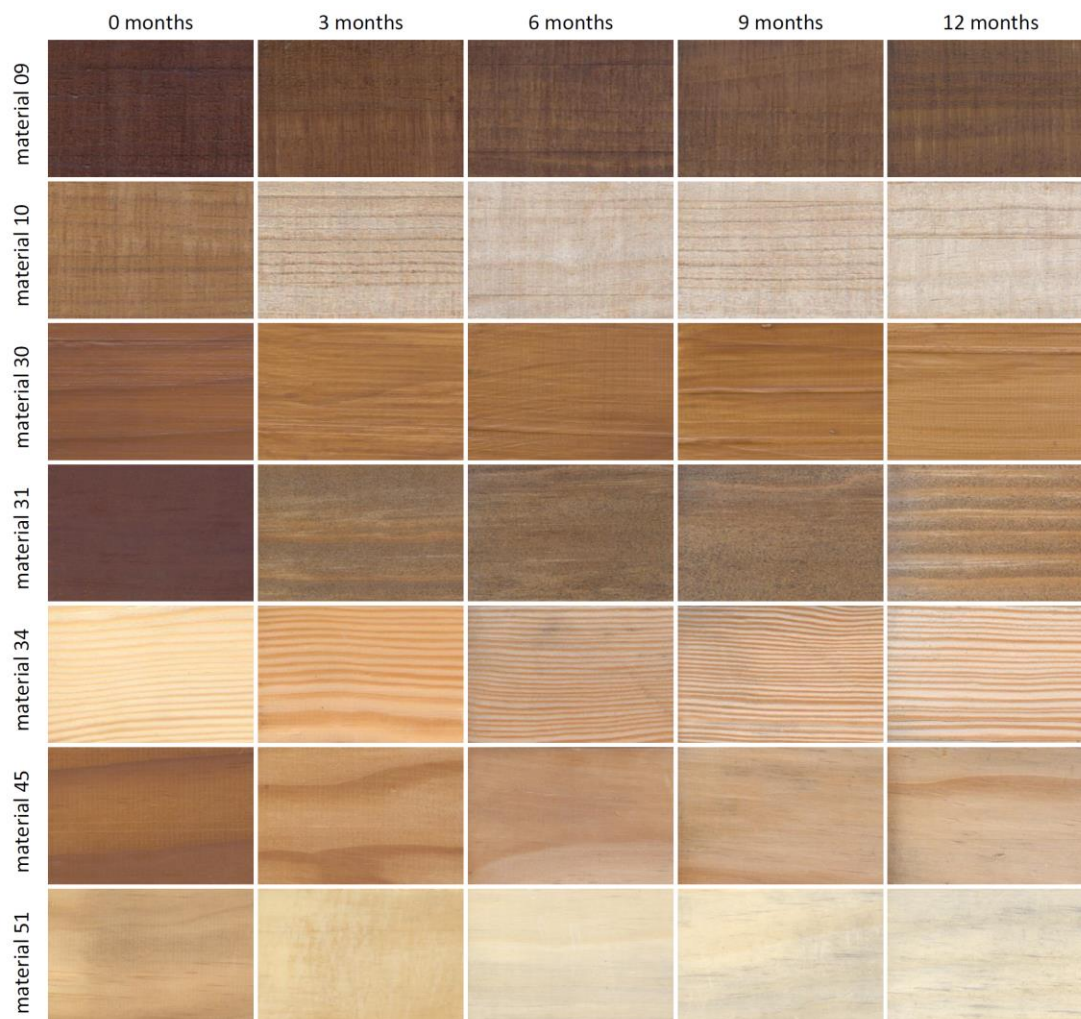
Figure 1: Change of samples appearance due to natural weathering in San Michele all'Adige (Italy)
