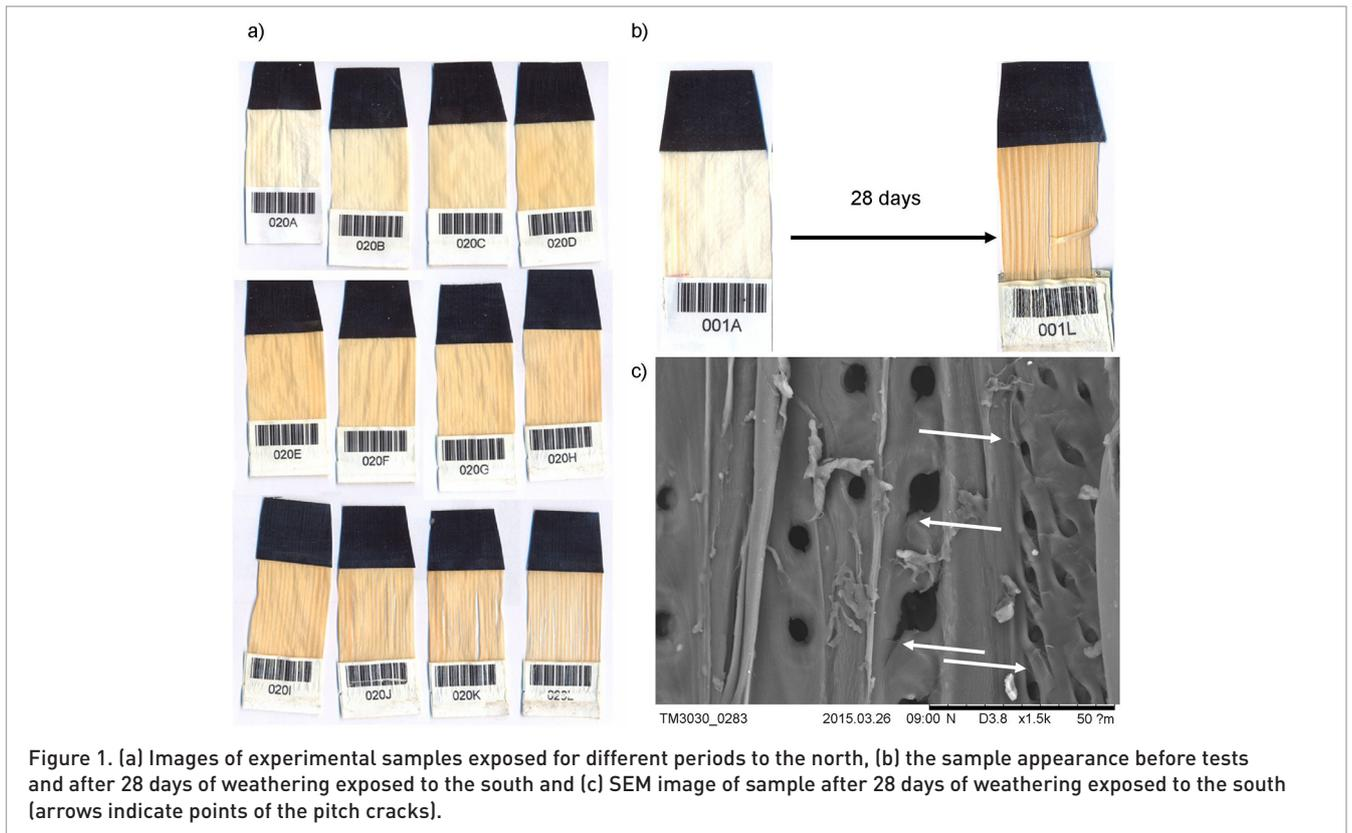
**Figure 1.** (a) Images of experimental samples exposed for different periods to the north, (b) the sample appearance before tests and after 28 days of weathering exposed to the south and (c) SEM image of sample after 28 days of weathering exposed to the south (arrows indicate points of the pitch cracks).
