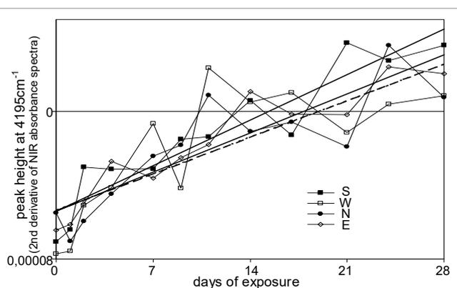
Figure 4. Kinetics of lignin changes (at  $4195\text{cm}^{-1}$ ) in relation to the exposure direction as recorded in NIR.
