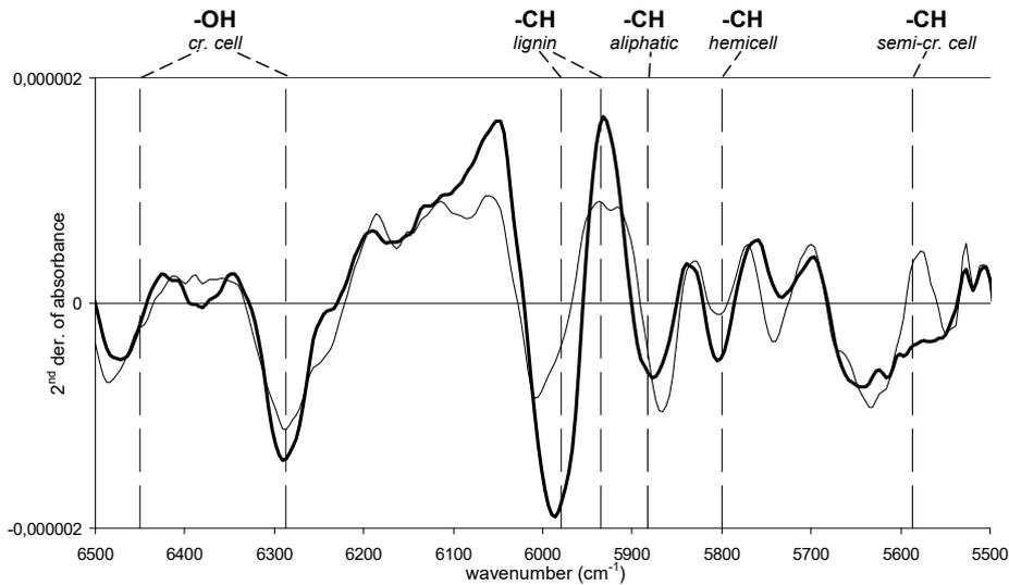
Figure 2. Second derivative of spectra of reference sample and wood weathered for 28 days.
