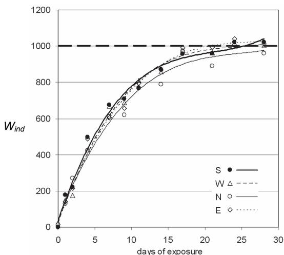
Figure 3. The weathering index rate  $W_{ind}$  predicted on the basis of PLS modelling of NIR spectra.
