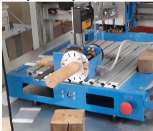
*Figure 2: Surface roughness scanner with Laser Displacement Sensor*
