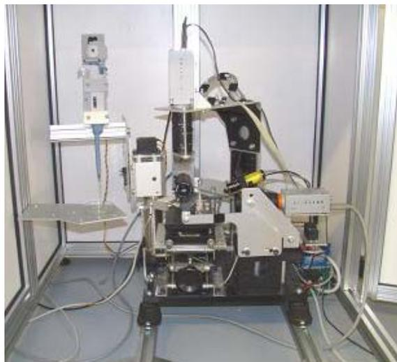
*Figure 3: Surface wettability scanner used for this experiments*
