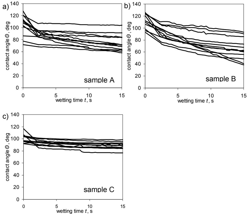
Figure 9: Dynamic contact angle of distilled water droplet placed on the particleboard panels of various types.
