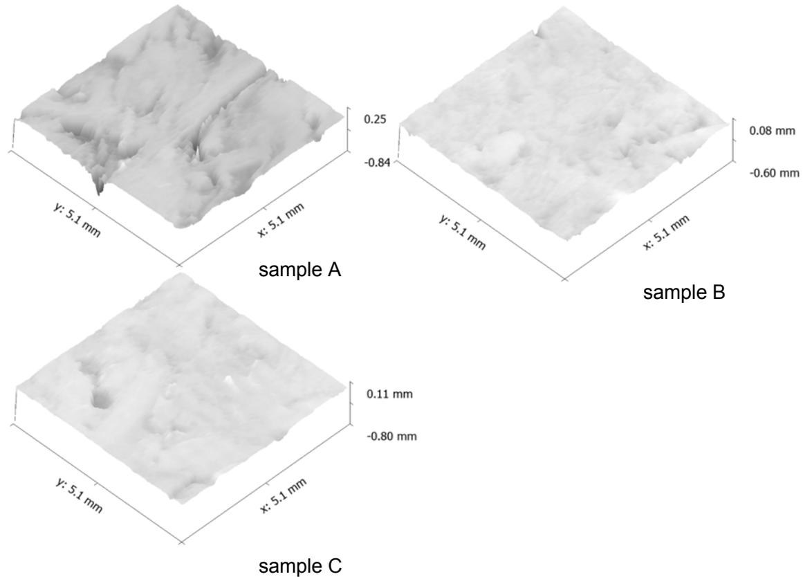
Figure 7: 3D surface roughness maps of particleboard panels type A, B and C
