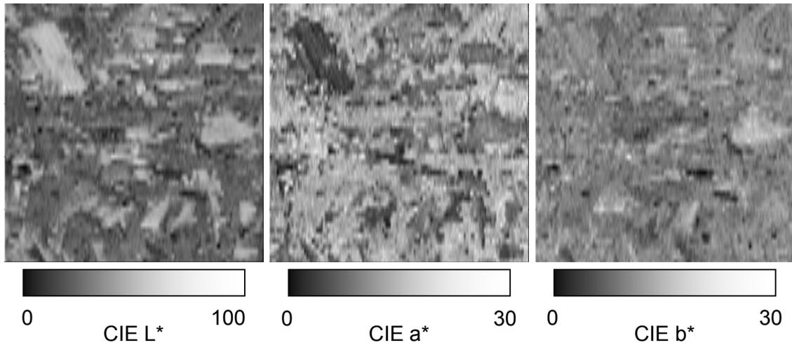
Figure 5: CIE Lab colour maps for  $L^*$ ,  $a^*$  and  $b^*$  components as measured on the surface of particle board panels with hyperspectral imaging
