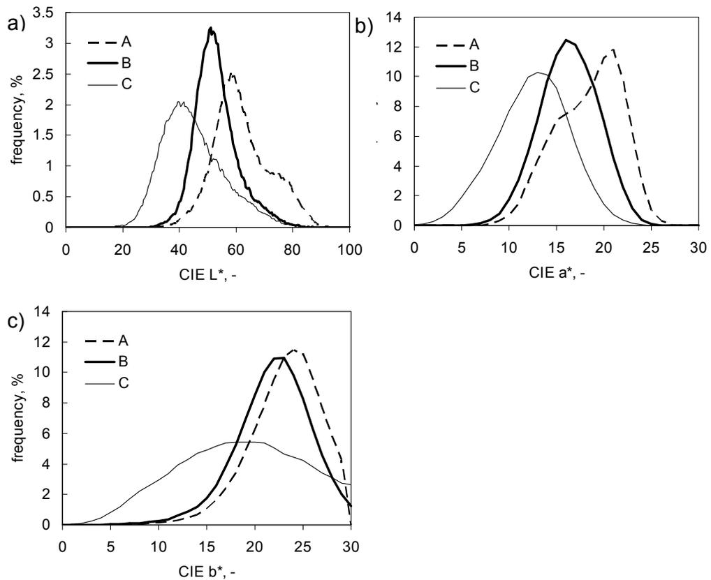
Figure 6: CIE Lab colour histograms for the tested samples of type A, type B and type C particleboard; CIE  $L^*$  (a), CIE  $a^*$  (b) and CIE  $b^*$  (c)
