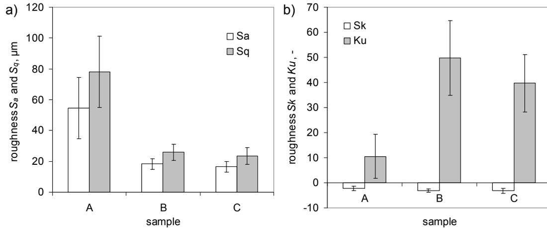
Figure 8: Surface roughness indicators as measured on experimental samples;  $S_a$ ,  $S_q$  (a) and  $S_k$ ,  $S_{ku}$  (b)
