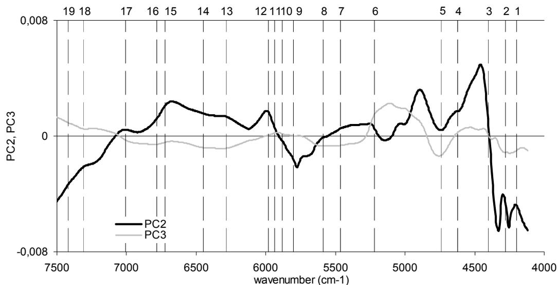
Figure 11: PCA model loadings for 2<sup>nd</sup> and 3<sup>rd</sup> components and spectral feature assignments
