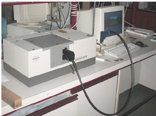
*Figure 4: Fourier transform near infrared spectrometer used for panels characterization*
