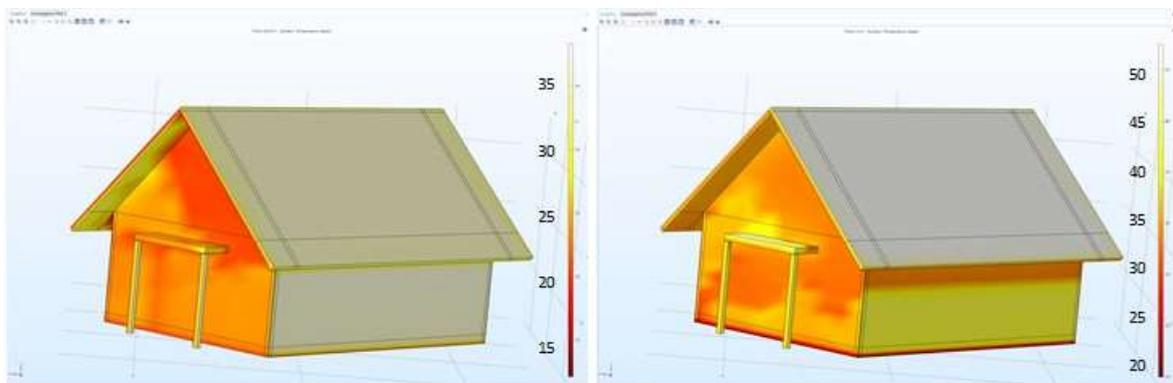
Figure 7: Simulation of surface temperature in January (left) and June (right).
