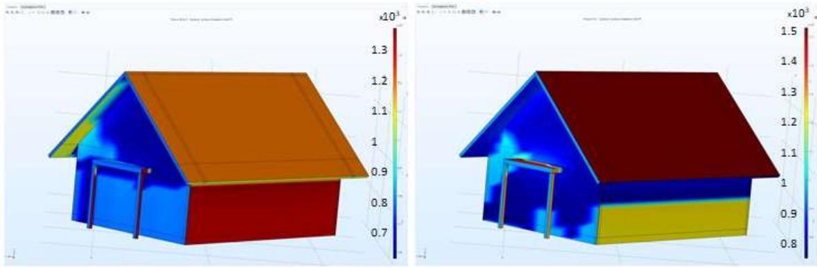
Figure 8: Simulation of surface radiation in January (left) and June (right).
