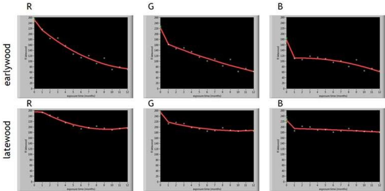
Figure 6: Curves of the RGB colour changes for early and latewood during one year of weathering.
