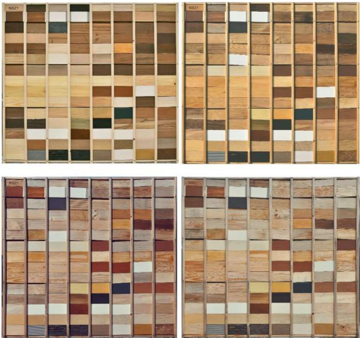
Figure 5: Experimental samples during natural weathering (southern exposure). Note: up, left: new samples set, up, right: 4 months, bottom, left: 8 months, bottom, right: 12 months of exposure.
