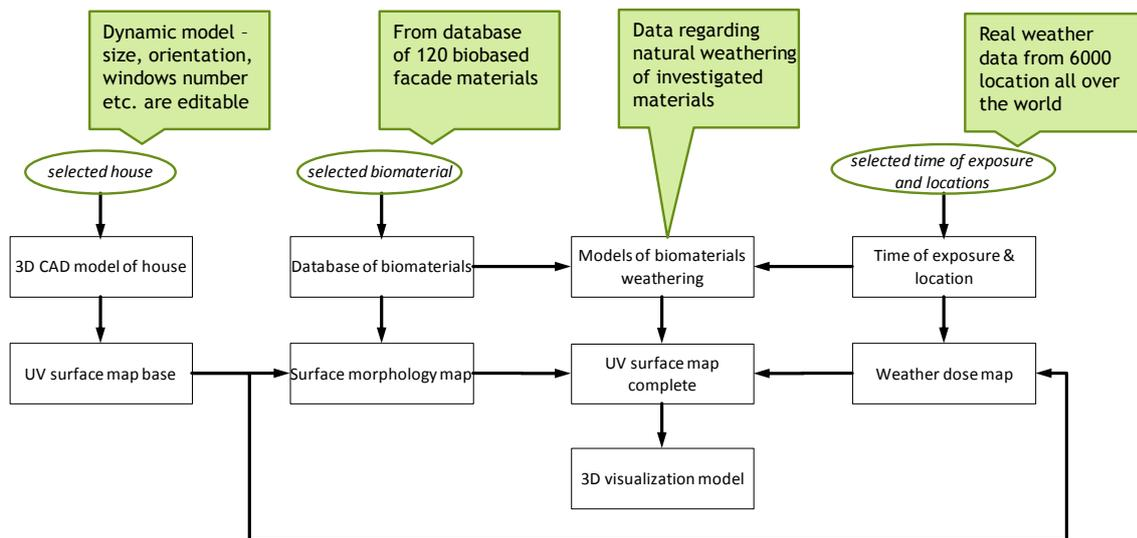
Figure 9: Software flow implemented within BIO4ever project (Sandak *et al.* 2017b)
