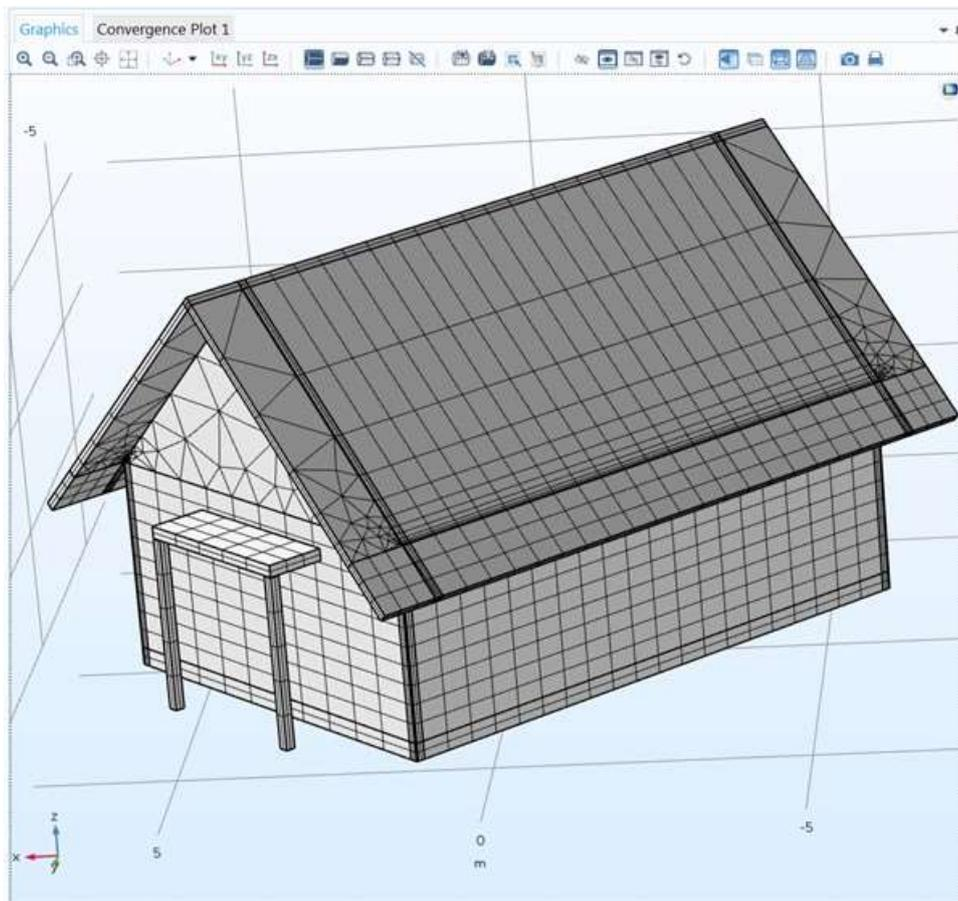
Figure 3: 3D model of the house with defined mesh as used for numerical simulation.
