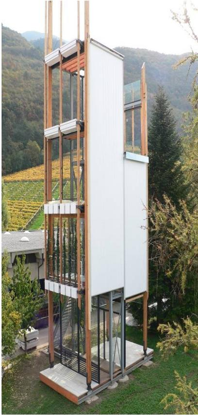
**Figure 2:** Prototype structure used to expose samples of investigated bio-materials to the natural weathering
