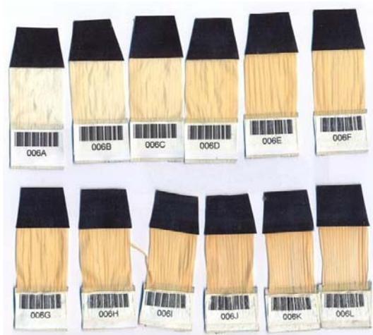
Figure 9: Appearance of samples after 1 month weathering test (western exposure)
