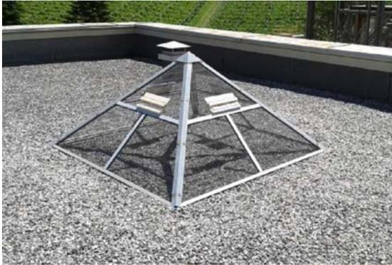
Figure 7: Experimental set-up for weathering test
