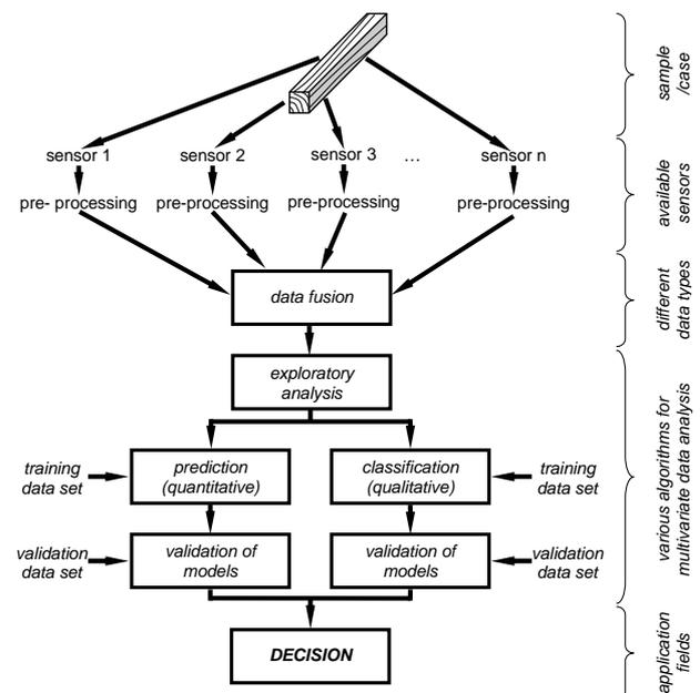
**Figure 6:** Multi sensor approach combined with multivariate analysis for assessment of timber structures [6]
