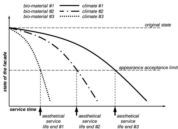
**Figure 11:** Models for aesthetical service life performance depending on bio-materials type and climatic loads.
