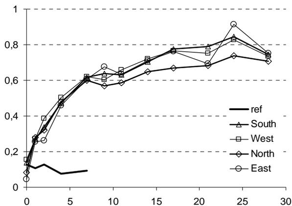
**Figure 10:** Progress of the weathering due to exposure duration (horizontal axis, days) and normalized components (vertical axis) used for computation of weathering index  $w_{ind}$ .
