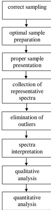
**Fig. 1.** Schema of proposed stages for wooden members characterization. Source: [10] modified.
