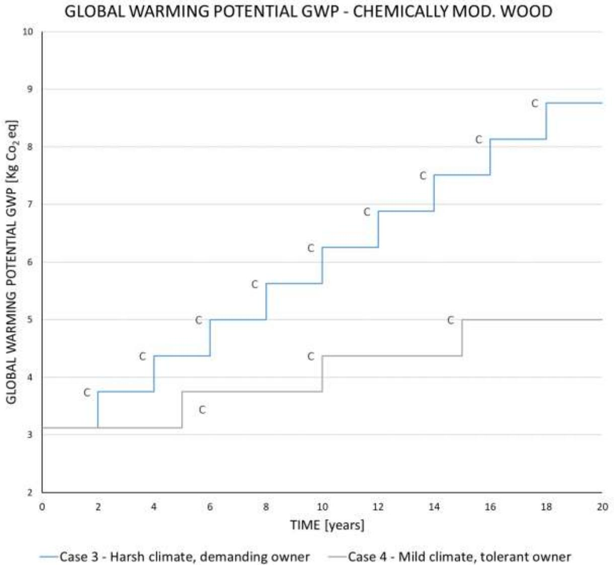
Figure 6: Global warming potential in 20 years of maintenance of a chemically modified wood façade in worst and best scenario. Capital letters indicate the different operations: “C” for cleaning
