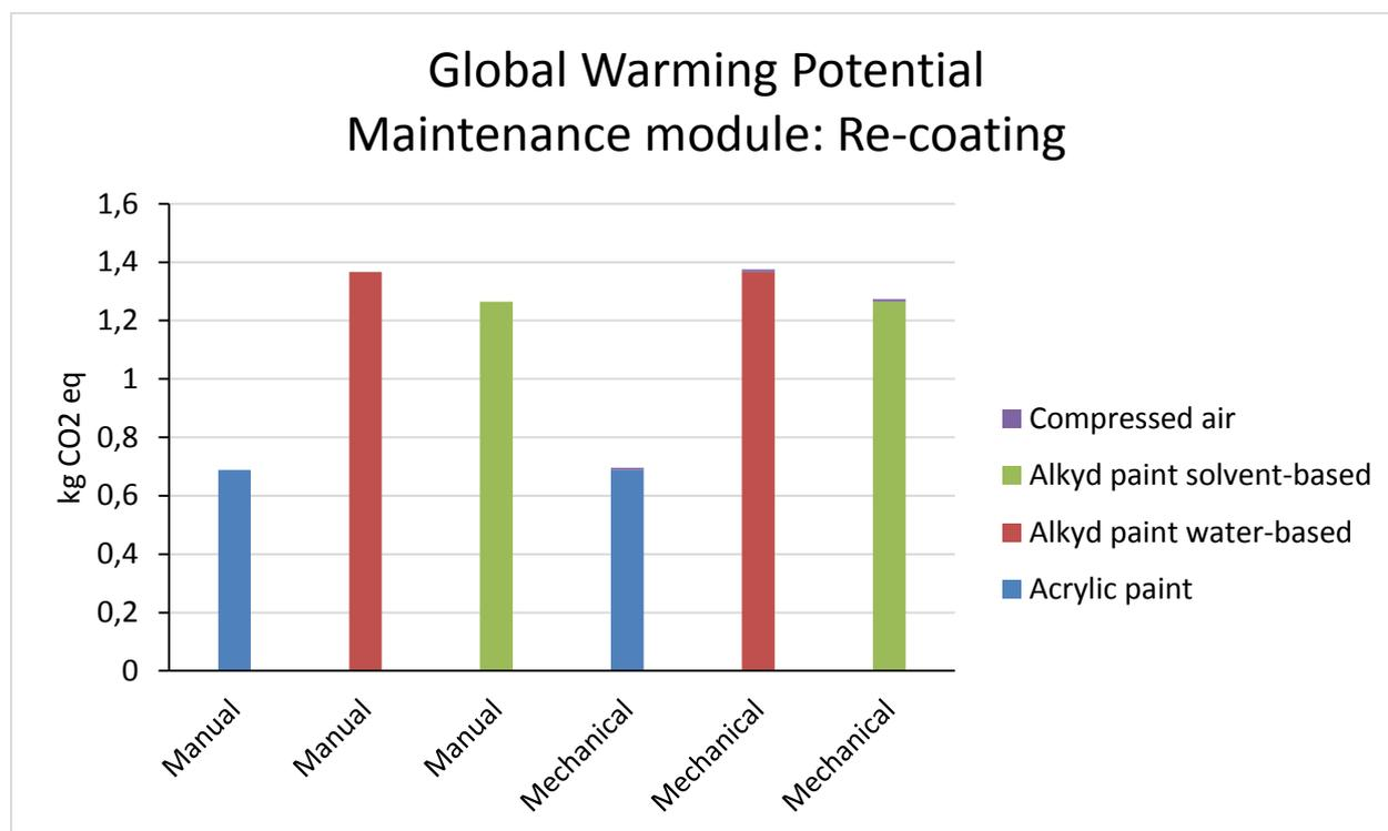
Figure 4: The graph shows, for six re-coating options, the contribution of each input and output to the Global Warming Potential expressed as kg of CO<sub>2</sub> equivalent.
