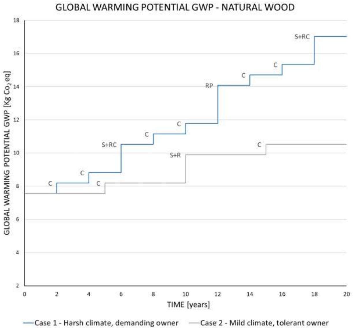
Figure 5: Global warming potential in 20 years of maintenance of a natural wood façade in worst and best scenario; Capital letters indicate the different operations: “C” for cleaning, “S+RC” for sanding and recoating, “RP” for replacement.
