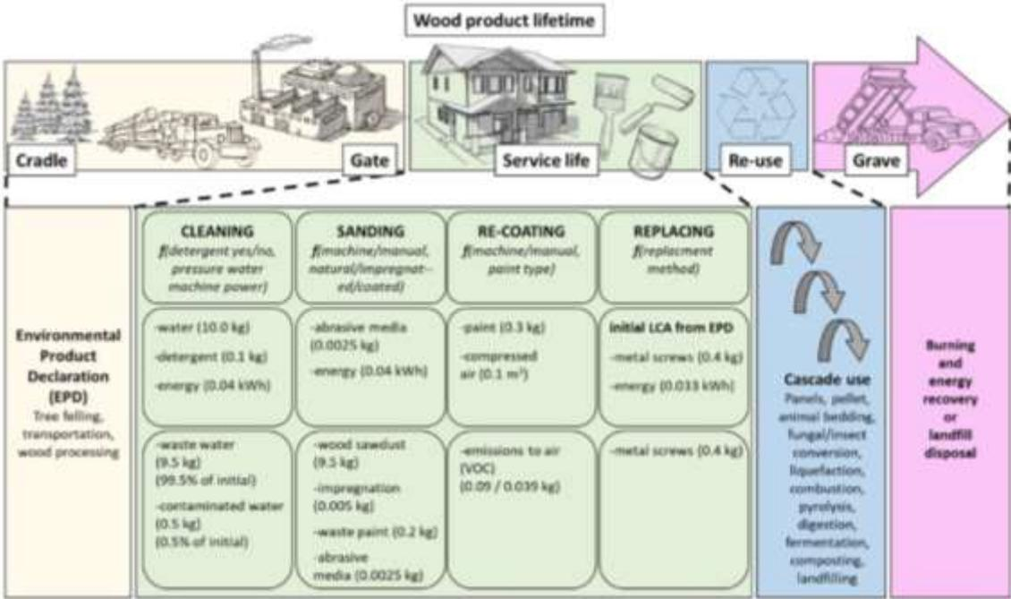
Figure 1: The modules considered for maintenance are: cleaning, sanding, re-coating, replacing. In brackets examples are given of the values for each input/output element for a functional unit of 1 m<sup>2</sup> of façade. These values can be determined directly by the user in the interactive LCA.
