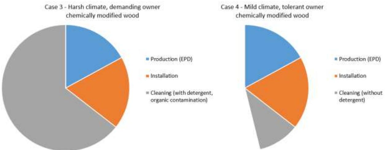
Figure 8: Relative share of the environmental impact (GWP) for the installation and maintenance operations of chemically modified wood façade in worst and best scenario.
