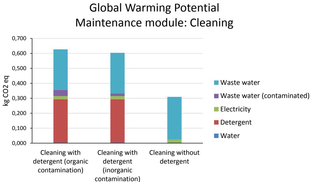
Figure 2: The graph shows, for three cleaning options, the contribution of each input and output to the Global Warming Potential expressed as kg of CO<sub>2</sub> equivalent.
