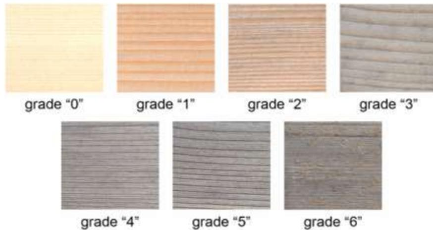
Figure 2: Weathered samples corresponding to seven levels grading scale
