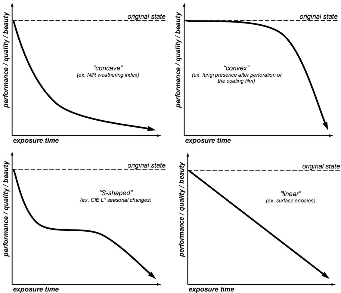
Figure 4: Various deterioration patterns observed in weathering of biomaterials
