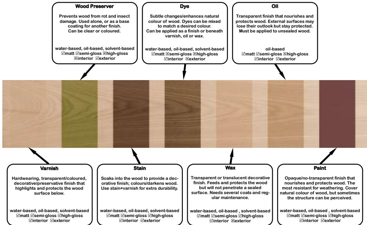
Figure 1: Appearance of wood after different finishing processes
