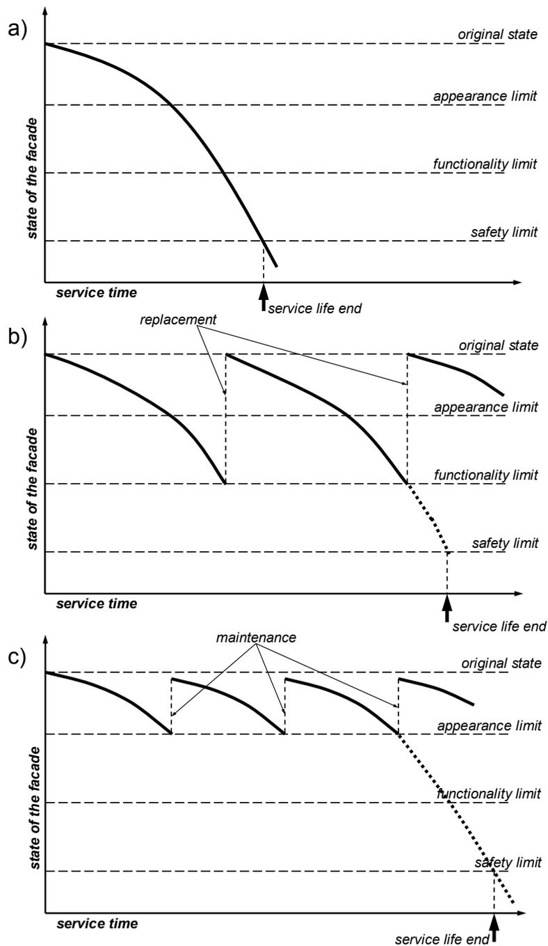
Figure 3: Estimation of the service life time according to different scenarios; no any repairs (a), replacement (b) and frequent maintenance (c)
