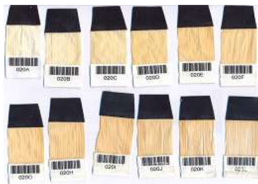
Figure 1. Thin samples appearance after weathering test (exposed against north)
