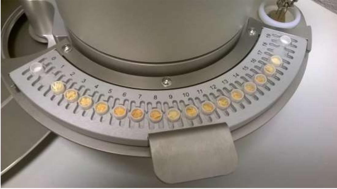
Figure 3: The samples cut into pieces of earlywood and latewood in the containers prior to the chemical analysis.
