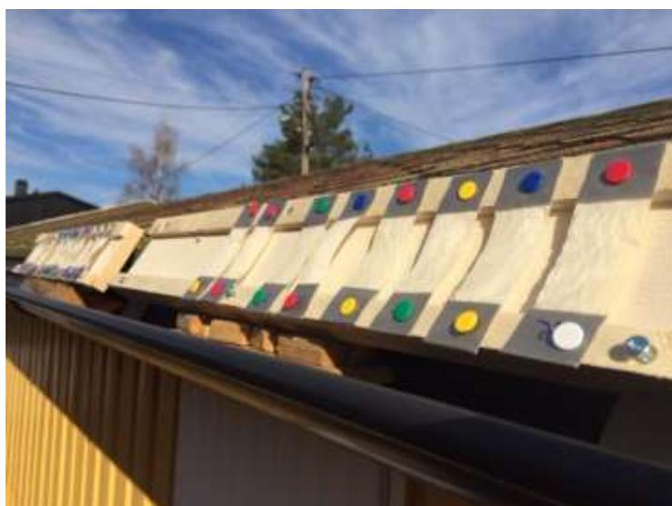
Figure 2: Thin samples exposed outdoors facing south.
