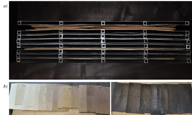
Figure 1: Veneers treatment set-up (a) and experimental samples after thermal treatment (b)
