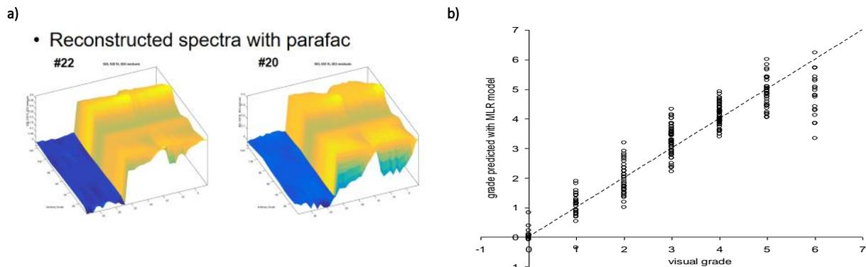
Figure 2: a) PARAFAC model of micro NIR results, b) MLR model of morphological characteristics and weather degradation visual grading
