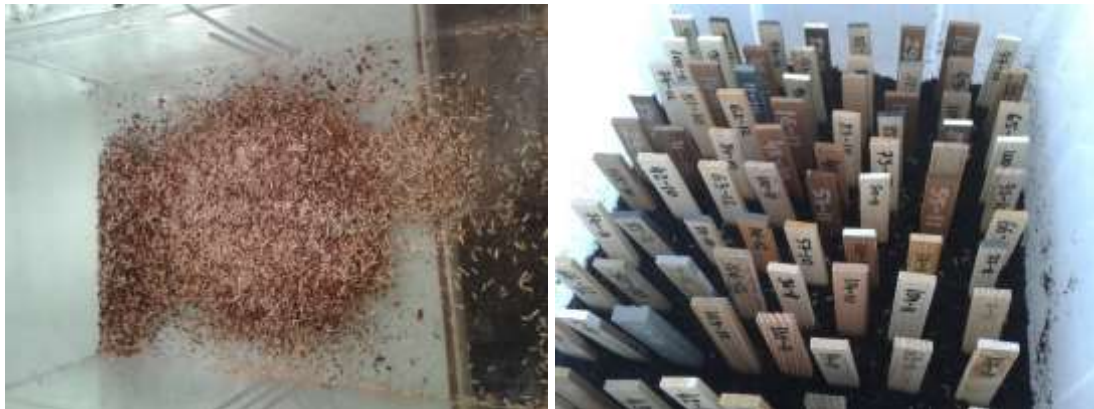
Figure 1: Termites extracted from the logs (left) and experimental samples at the start of the test (right)
